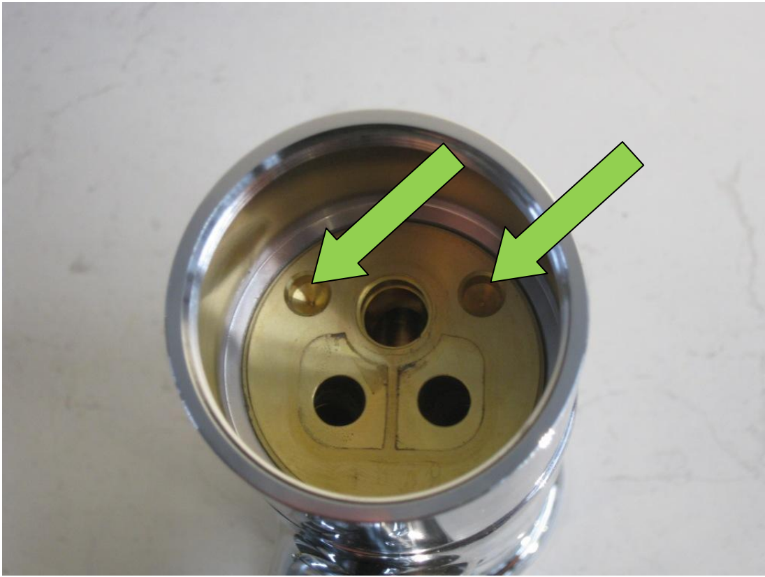
8a showing lug holes
